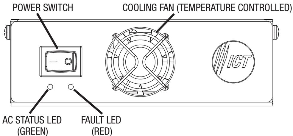
**Figure 2: ICT Inverter Back Panel**
