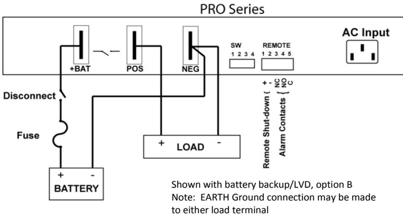
Connection Diagram (Showing Rear Connectors and SW Switch 1-4)
