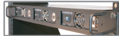
Three Site Inverter 300 units mounted on a single 1RU 19-inch rack provides 900 watts of power and six AC outlets.
